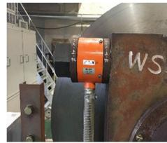
Figure 2: Load cell.
