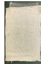
Figure 3: Side dam strip.
