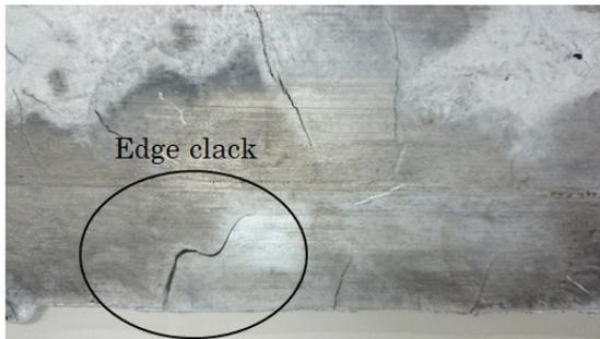
Figure 7: Produced strips (roll speed 30m/min).
