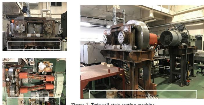
Figure 1: Twin roll strip casting machine.
