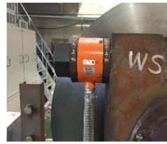
Figure 2: Load cell.
