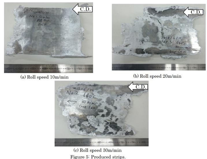
Figure 5: Produced strips.
