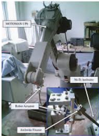
Figure 5: Archwire bending robot based on MOTOMAN UP6.
