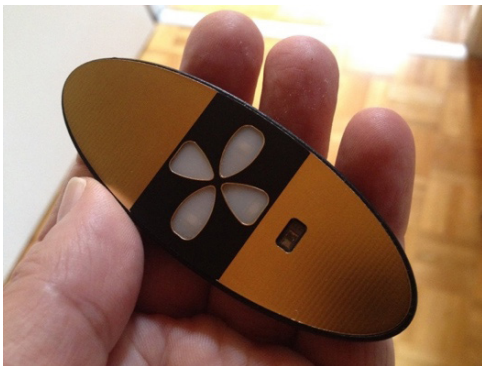
Figure 2: The SATHeart device can measure photoplethysmogram in a convenient way. The algorithms extract parameters from the pulse wave, among them the vascular stiffness and pulse wave velocity.
