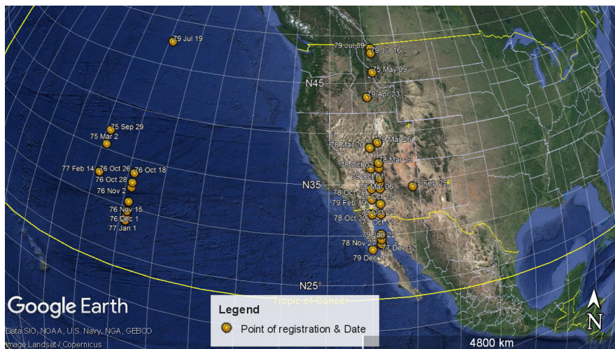
Figure 19: Points of registration of pulses of alpha particles with a flux of not less than 1000.\text{cm}^{-2}.\text{s}^{-1}.\text{sr}^{-1}.\text{MeV}^{-1} in the western parts of the USA, as well as in the eastern Pacific. A Google Earth map was used.
